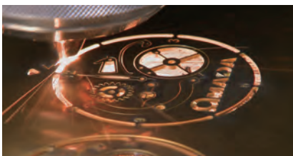
Processing copper (highly reflective material) with a fiber laser machine
