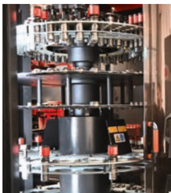
The AMADA EML-2515AJe is equipped with a PDC tool changer which changes over punches and dies fully automatically.
