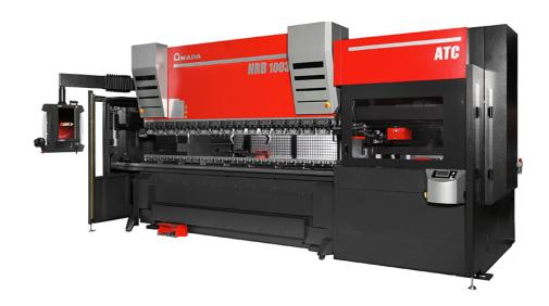
With over 300 ATC (Automatic Tool Change) press brakes installed throughout Europe and more than 1000 globally, AMADA is bringing the company's unique ATC technology to its mid-range line-up for the first time. Previously only available on high-end press brakes such as the AMADA HG-ATC and its predecessor the HD-ATC, the new AMADA HRB-ATC midrange model responds directly to market demand for a solution of this type using original AMADA tooling.
