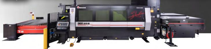
In terms of sheet profiling, around 90% of capacity at NIJEN is used to process stainless steel up to 15mm thick, and 10% for cutting aluminium up to 12mm. With regard to tube processing, the company cuts material up to 154mm diameter, in 6mm wall thickness. NIJEN makes full use of both shuttle tables, as well as the RI unit. Typical batch sizes are 80-150, although sometimes up to 500.
