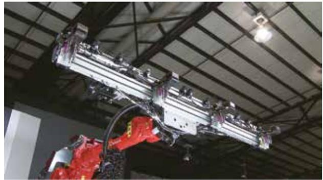
*These two grippers are dedicated to rib part and they allow processing of complex shapes with shorter cycle times.*
