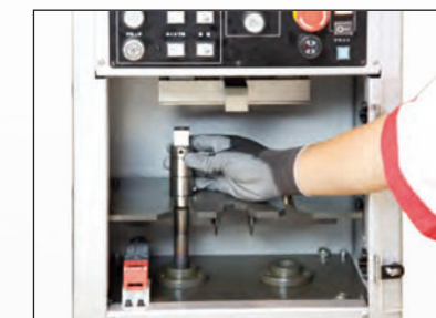
② Setting the tool on the measuring unit
