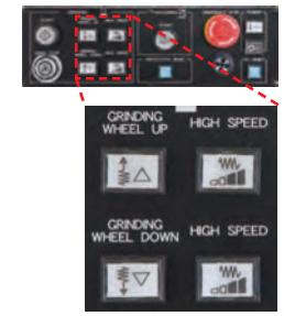
③ Depress start-button after lowering the wheel near the tooling
