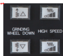
Depress start-button after lowering the wheel near the tooling
