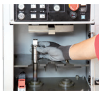
Setting the tool on the measuring unit
