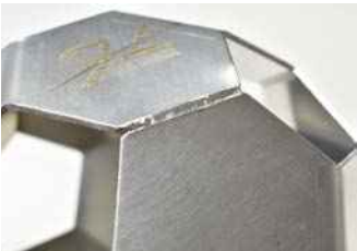
Laser welding of stainless steel (SUS) sheets
